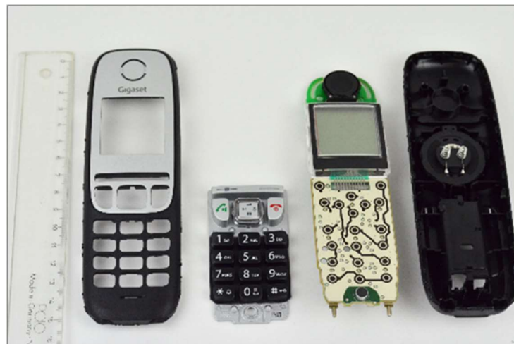
13 Figure 47 : Cordless phone handset teardown – frontside cover, key pad, 14 display and mainboard, backside cover
