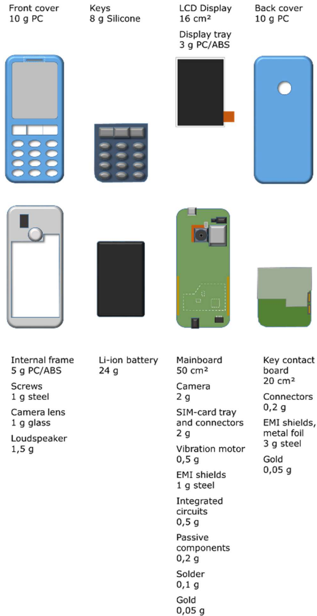
7 Figure 25 : Feature phones – major parts, materials and weights
