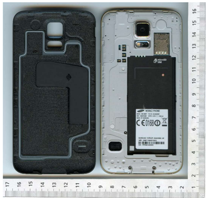
24 Figure 66 : Samsung Galaxy S5, backside cover removed
