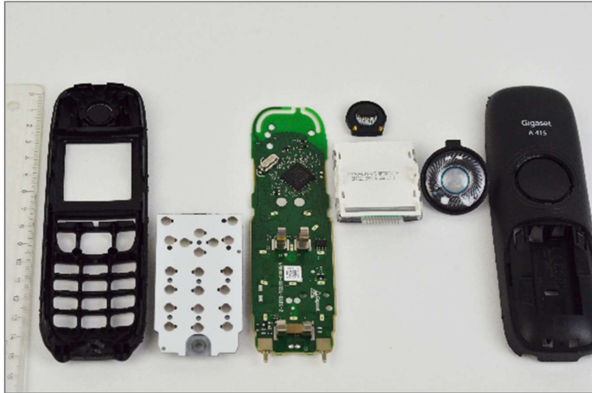
2 Figure 48 : Cordless phone handset teardown – frontside cover inside view, 3 key pad backside, mainboard reverse side, display unit backside view, 4 loudspeaker, backside cover
