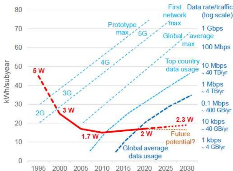
**Figure 32: Average power, electricity use and data per mobile subscription over time for mobile access networks (Malmodin 2020)**
