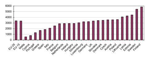
Using the degree-days as a parameter, we can also make an estimate of what used to be called the <u>heating season</u>: Heating season in hours = (degree-days + 2000). Heating season in months = rounded ( $12^*$  heating season in hours/8760).
