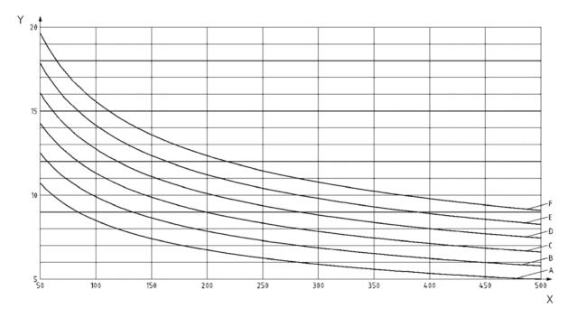
**Figure 3-1.** PrEN 15332: Suggested A-G labeling classification for hot water storage tanks on the basis of the standby loss related to the hot water capacity in (Wh/I)/d [=Y axis] and the storage capacity in litres [= X axis]. A similar graph exists for capacities 500-2000 litres.
