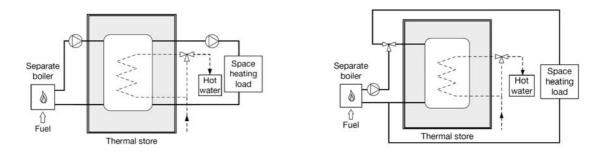
Figure 2-3. Integrated Thermal Store (left) and 'Hot water only' Thermal Store (right)
