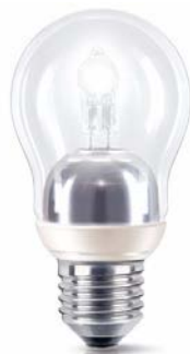
Figure 3b. Non-directional mains voltage halogen lamps class B. This lamp was brought on the market in a 20 and 30 Watt version by Philips in 2008. Philips production stopped in 2010, reportedly for lack of commercial success. The retail price was € 9.95 and declared life time 3000 h. The lamp was fully dimmable. A voltage transformer was incorporated in order to host a class B low voltage halogen lamps (figure 2b). Currently Chinese-made lamps exist with similar design (i.e. with transformer), similar price and –as far as could be assessed– similar lack of commercial success; it could not be ascertained whether these lamps meet the class B requirements.
