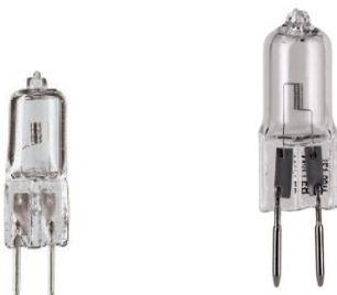
Figure 2a. Non-directional low voltage halogen capsules class C. Caps: G4 (left), GY6.35 (right). Common power range from 6 to 75 W. Common voltage range: 6-48 V (most popular: 12 V and 24V). Rated product life 1500-4000 h (to be restricted to \geq 2000 h after 1.9.2013). Prevalently used with external reflector in spot-lights (ceiling, furniture, etc.), desk-lamps and small decorative lamps. Declared as energy label classes ‘C’. Consumer list prices of A-brands, including tax, up to € 3.5 per unit (class ‘C’) or € 4.5 per unit (class ‘B’). Street prices of grey-brands, including tax, as low as € 1.1 per unit (class ‘C’).
