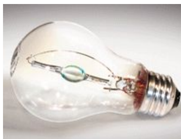
Figure 12. E26 halogen lamp 21 with double-ended halogen capsule and infrared coating (120 VAC, 50 Watt, 1600 lm)
