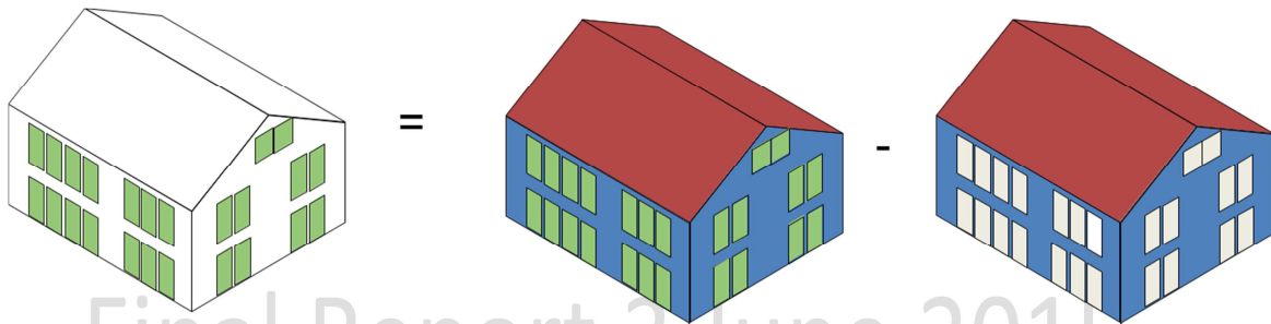
Figure A 57 Visualisation of calculation procedure for window energy performance
