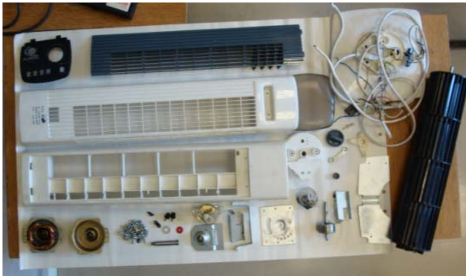
Figure 4-4: Disassembly photo of fan 2 (Tower Fan)
