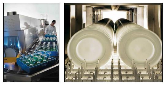
Figure 7 Principle of a basket conveyor dishwasher (left) and a belt conveyor dishwasher (right)
