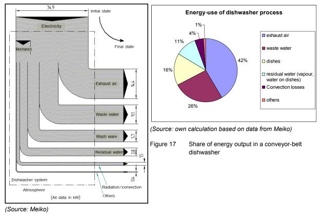
Figure 16 Energy in- and output of an exemplary conveyor-typedishwasher
