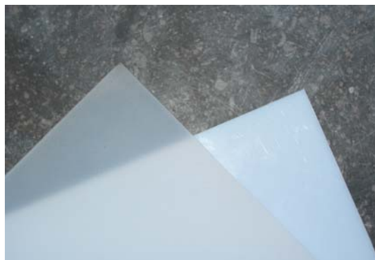
Figure 6-8: Left satinated PMMA and right white colouration PMMA diffusor material
