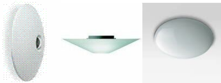
Figure 6-9: Luiminaire(left) having LOR = 83 with special finish on the PMMA screen for direct&indirect lighting Luminaire (middle) with LOR = 70 having a glass diffuser with satin finish for direct lighting versus Luminaire (right) with LOR =62 having a white colouration PMMA screen for direct lighting
