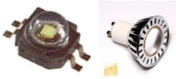
Figure 6-4: Typical WLED component and LED lamp
