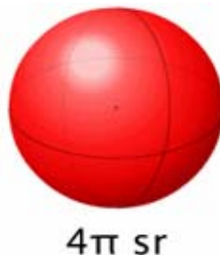
Figure 1-1: Visualization of a complete solid angle.
