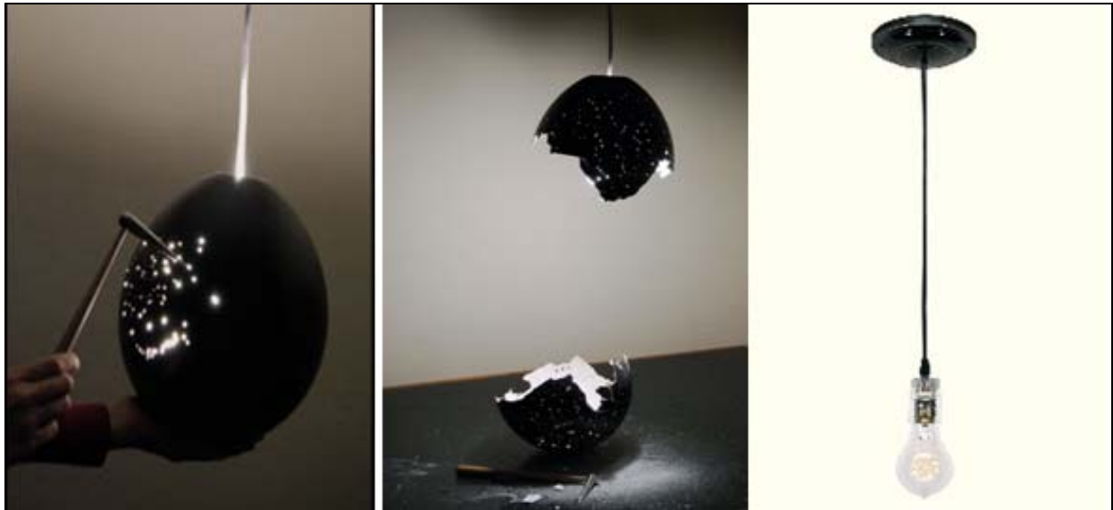
Figure 3-2 Domestic luminaire for NDLS: left with LOR <0.1, middle 142 LOR > 0.5, right >0.99
