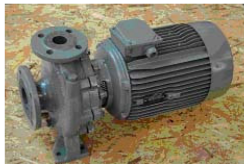
Figure 1-9 End suction close coupled design of single entry volute pump (Flowserve)
