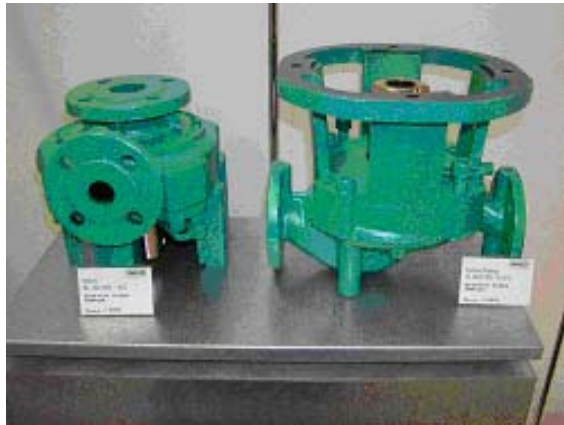
Figure 1-10 End suction and in line pumps, with outlet at right angle and in line respectively. The motor is connected to the bottom and top respectively. (Wilo)
