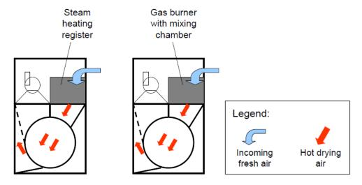
Figure 33 Heating systems of dryers 44
