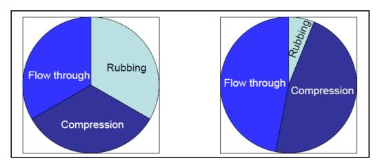
Figure 21 Components of the mechanical action: oscillating washing action and rotating washing action
