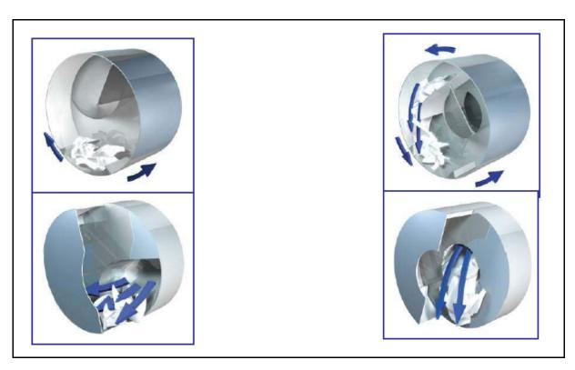
Figure 20 Oscillating drum movement (left side) and rotating drum movement (right side)
