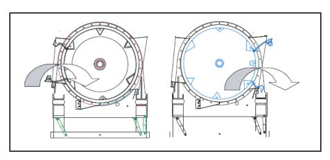
Figure 12 Drum Design: Open Pocket
