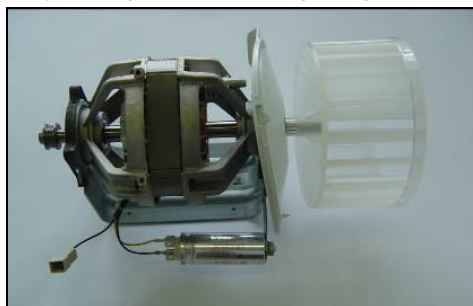
Figure 85: Motor and fan 37
