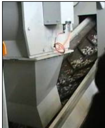
Figure 125: B- The heavy part falls on the treadmill
