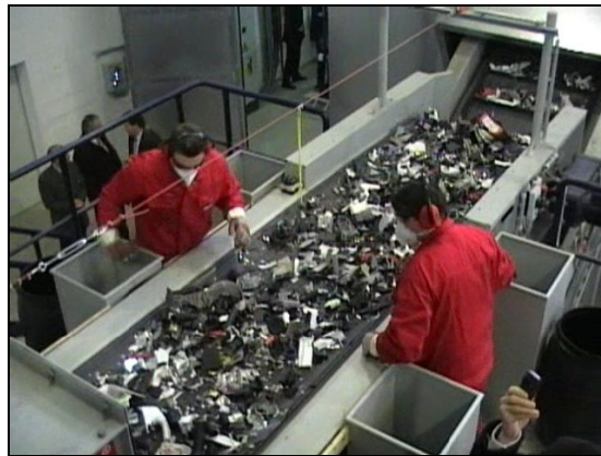
Figure 122: Cleaning up of shredded equipment
