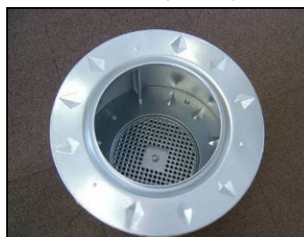
Figure 97: Drum of a compact tumble dryer 51
