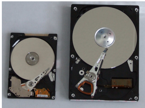
Figure 6-2: HDD for STBs (standard 3.5” –right; compact 2.5” –left)
