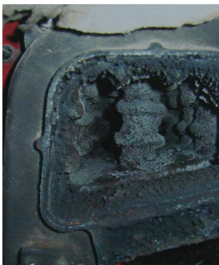
**Figure 3-13: Soot and tar fouling of heat exchange surfaces**
