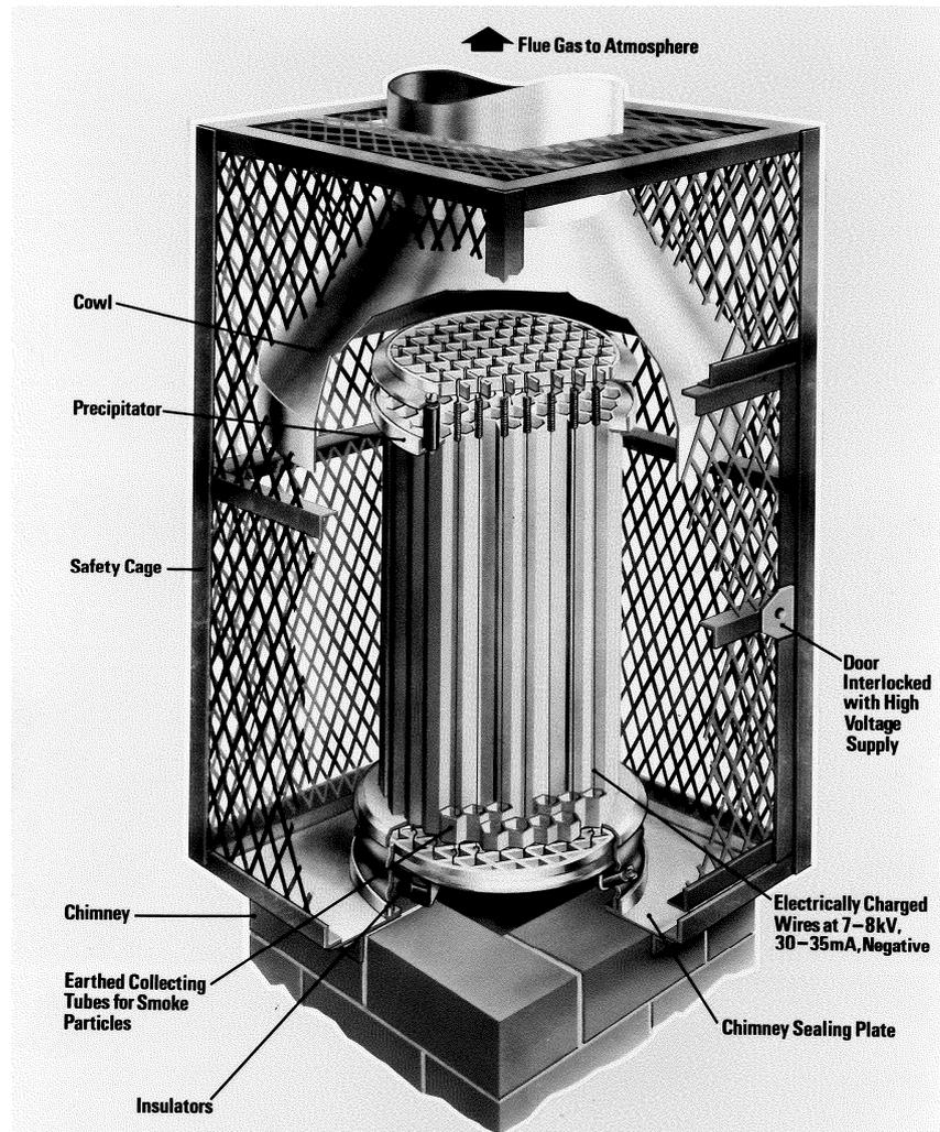
**Figure 1-20: Smoke measurement by electrostatic precipitator<sup>42</sup>**
