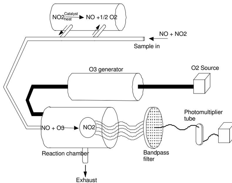
Figure 1-14: Example of arrangement of a chemiluminescence analyser<sup>35</sup>
