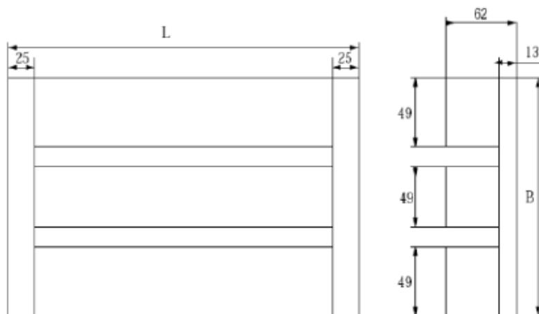
Figure 1-17: Arrangement of the standard test fuel
