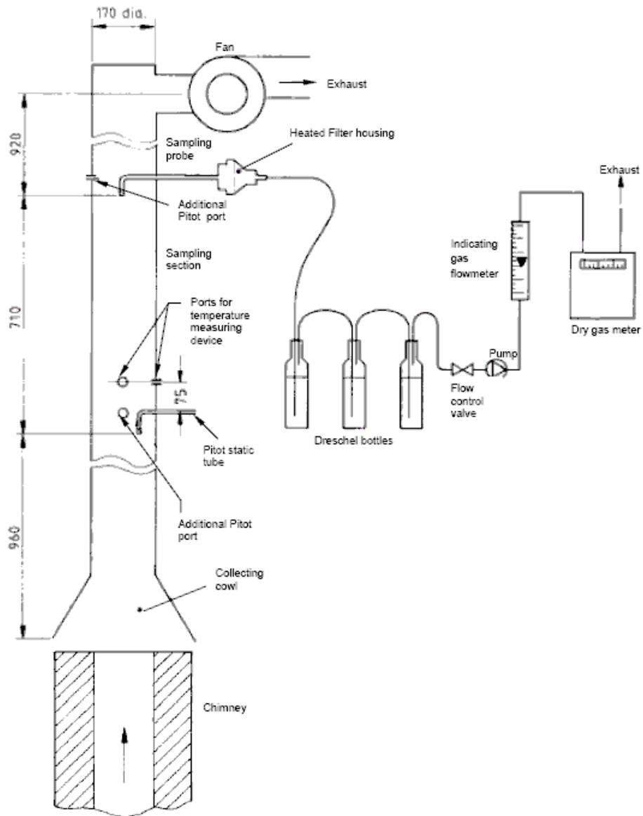
Figure 1-21: General arrangement of dilution tunnel and sampling train<sup>43</sup>
