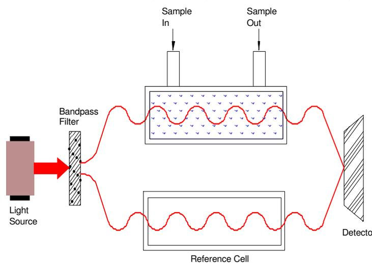
Figure 1-15: Example of a NDIR analyser<sup>36</sup>
