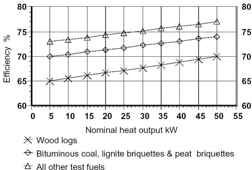
Figure 1-24: Boiler efficiency, according to EN 12809
