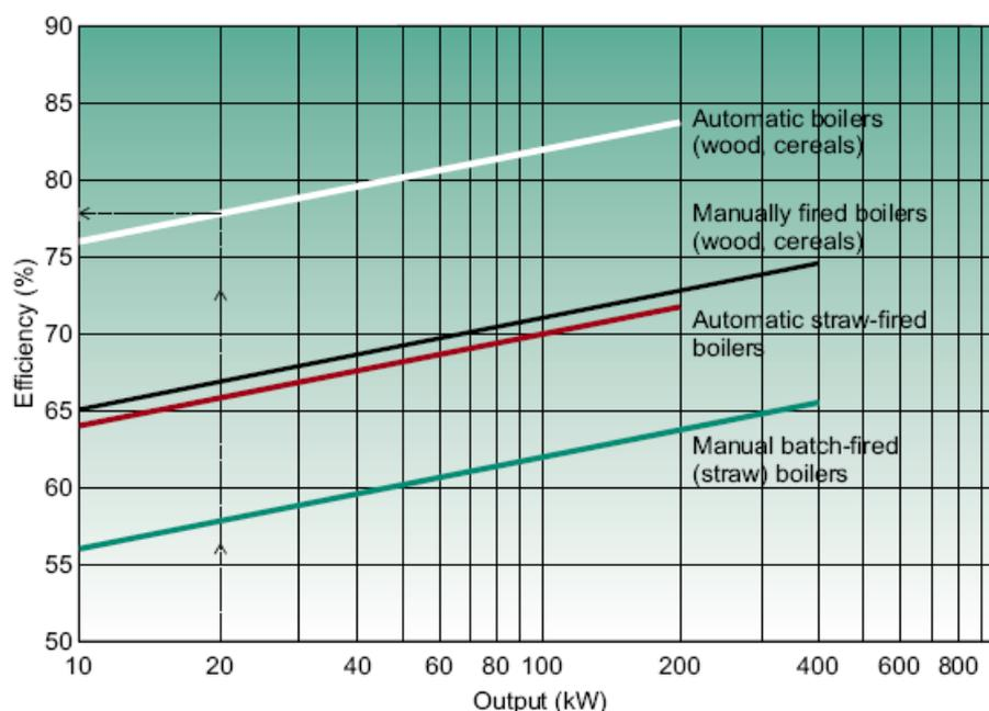
**Figure 1-23: Danish subsidy scheme minimum efficiency requirements for small biofuels boilers, according to the type of appliance**
