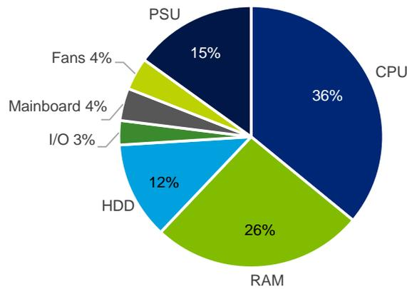
**Figure 19: Single CPU server energy distribution at maximum load**
