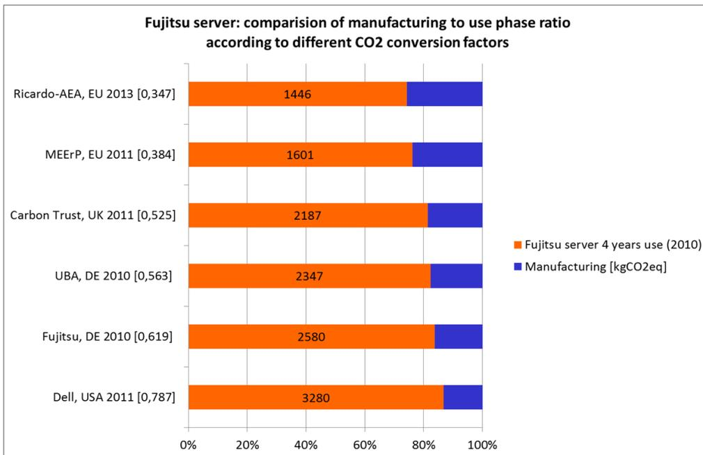
**Figure 2: Calculation of the Fujitsu server PCF with different CO<sub>2</sub> conversion factors**
