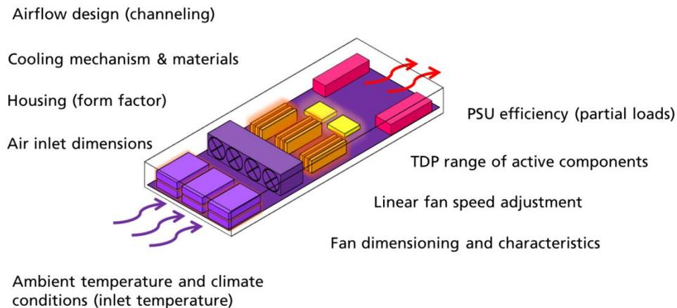
**Figure 20: Thermal design elements of servers and data storage equipment**
