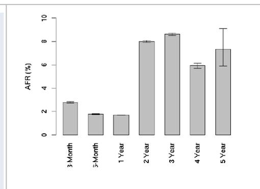
Figure 30: Annualised failure rates broken down by age groups<sup>36</sup>
