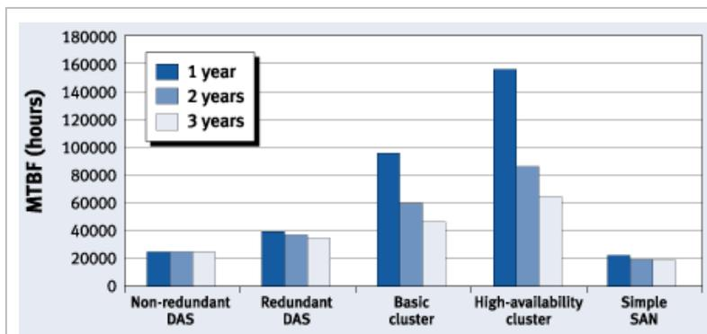
Figure 29: Comparison of MTBF over three years, for different configurations<sup>35</sup>
