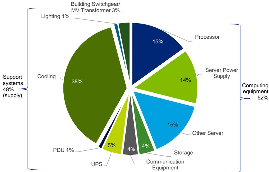
Figure 27: Average distribution of power consumption in a data centre in 2010 (Source: Emerson Power)<sup>30</sup>
