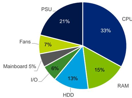
**Figure 18: Single CPU server energy distribution at idle level**
