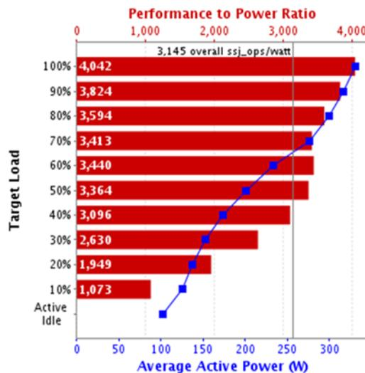
Figure 16: Example of a SPECpower assessment result (2012)
