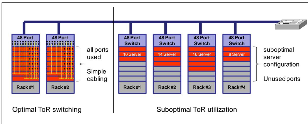
Figure 25: Top-of-Rack switching
