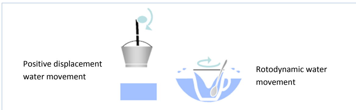
Figure 1-1: Operating principles of positive displacement and rotodynamic water pumps
