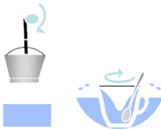
Figure 1-1: Operating principles of positive displacement pumps (pump on left side) and rotodynamic water pumps (pump on the right side)
