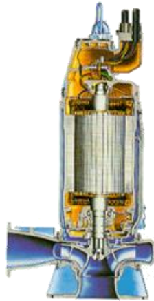
Figure 1-12: Cutaway of a Submersible Pump showing the motor integrated with the impeller.
