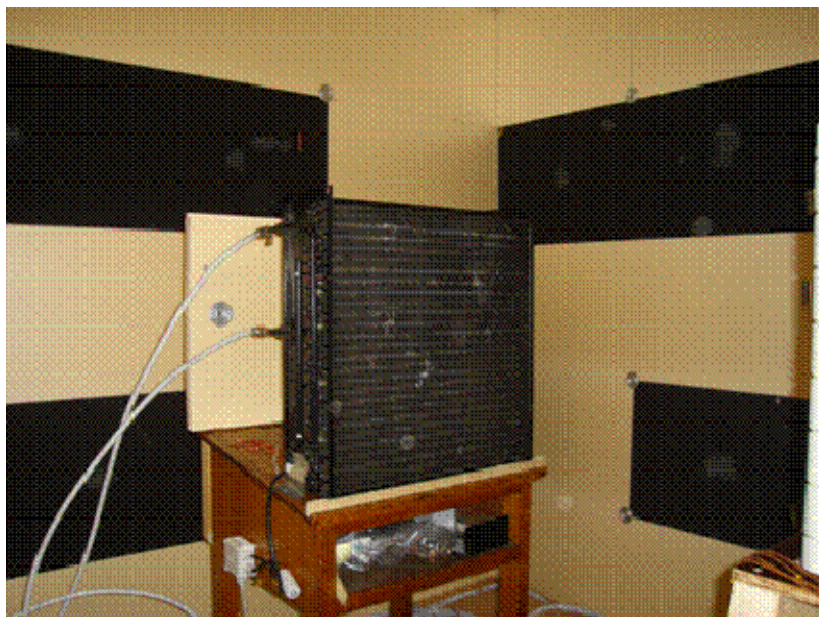
Figure A.2: The cooling-coil of the outdoor calorimeter
