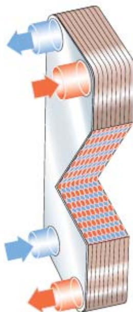
Figure 4-17: Plate heat exchanger principle, source Alphasval
