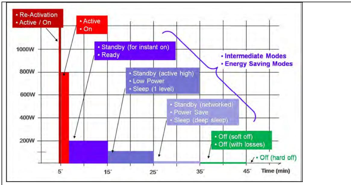
Figure 7: Common mode structure and mode terminology
