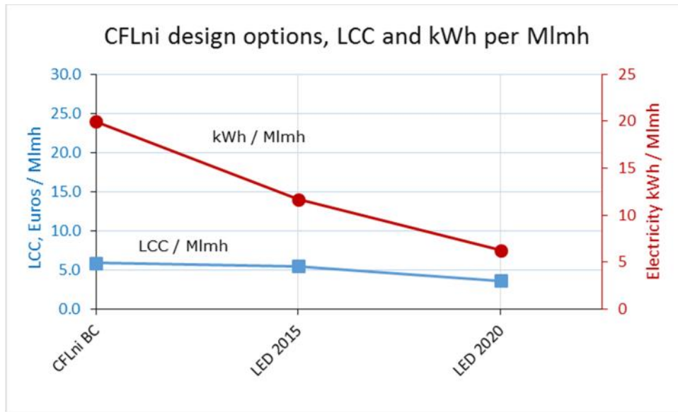
Figure 9 Design options for CFLni: life cycle cost (LCC, in euros/Mlmh, blue line with square markers, axis left) and electricity consumption (in kWh/Mlmh, red line with round markers, axis right). See Table 6 for underlying data.
