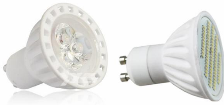
Figure 42: Narrow beam DLS with high-power LEDs and lenses (left) and wide beam DLS using a string of mid-power LEDs (right).
