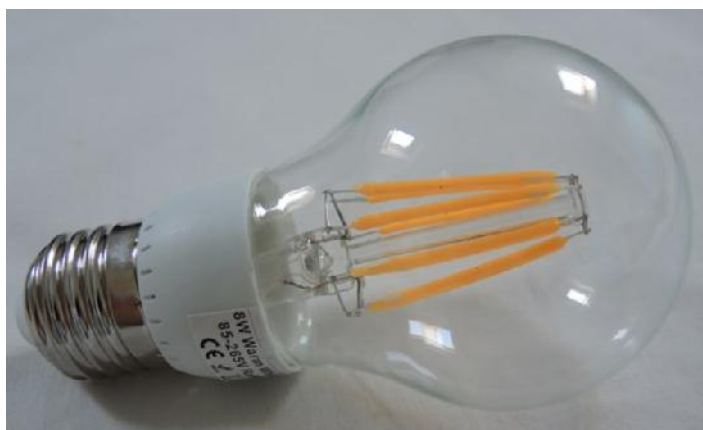
Figure 39 Example of an AC Mains-Voltage Non-Directional LED Filament Lamp. For test data on these lamps and for details on technology and manufacturing see the source 226 .
