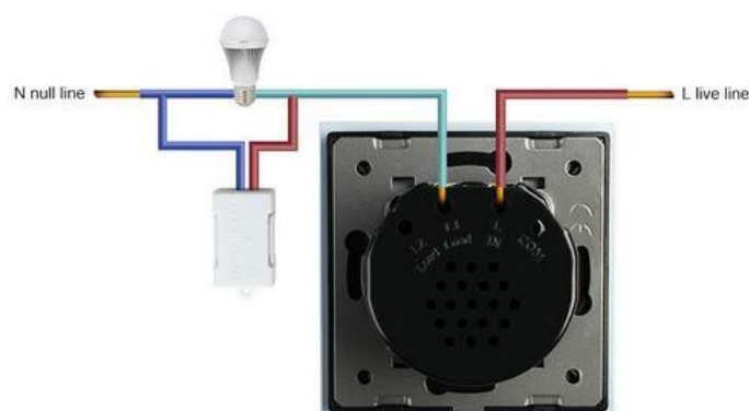
Figure 17: External adapter installed parallel to the lamp to enable switches and dimmers in 2-wire circuits as illustrated (source: Livolo 85 ).
