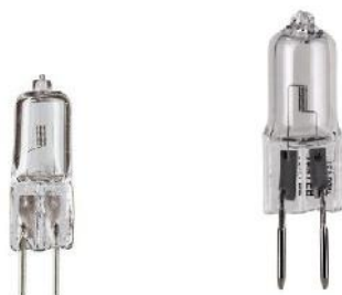
Figure 31: Non-directional low voltage halogen capsules class C. Caps: G4 (left), GY6.35 (right). Common power range from 6 to 75 W. Common voltage range: 6-48 V (most popular: 12 V and 24V). Rated product life 2000-4000 h. Prevalently used with external reflector in spot-lights (ceiling, furniture, etc.), desk-lamps and small decorative lamps. Declared as energy label classes 'C'. Consumer list prices of A-brands, including tax, up to € 3.5 per unit (class 'C') or € 4.5 per unit (class 'B'). Street prices of grey-brands, including tax, as low as € 1.1 per unit (class 'C'). (Source: Stage 6 review report 217 )
