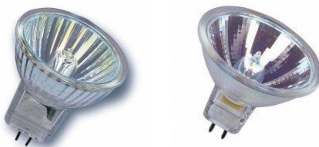
Figure 29 Examples of low voltage halogen reflector lamps. Left: argon filled class C lamp (now phased out by regulation 1194/2012); right: xenon filled class B lamp with infrared coating and dichroic reflector.
