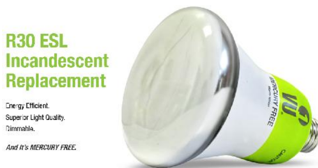
Figure 3 ESL lamp from VU1 Corporation. R30 Reflector for use in place of standard 65W incandescent R30 bulbs for recessed light fixtures. Declared characteristics: 500 lm, 19.5 W, 115 V AC, CCT 3200 K, CRI 90+, power factor >0.99, life 11,000 hours without significant colour shift, full dimming (triac), illuminance (at 1m) in Cooper Halo™ recessed luminaire: 0° 180 Lux, 45° 138 Lux, 60° 103 Lux, price: $15 / piece (source: http://www.vu1corporation.com/ )
