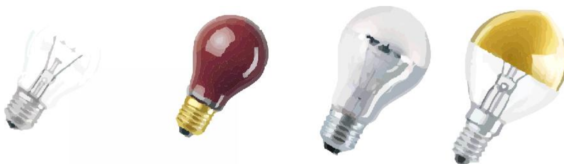
Figure 41 Classic and decorative incandescent lamps. From left to right: 1) Classic A-shape incandescent lamp, 230V, E27. Manufacturer website: Only 15W version can be supplied in the EU, the higher wattages are marked 'non EU'. 2) Decorative Colour A-shaped incandescent lamp, 11W, 27 lm, 230V, E27. Application: party lights, fair and amusement parks (merry-go-round, etc.). 3) Two decorative ant-glare incandescent lamps, 40-60W, 570lm, 230V, E27/E14. Applications: Mirror-lamps, theatre and barber shop mirrors
