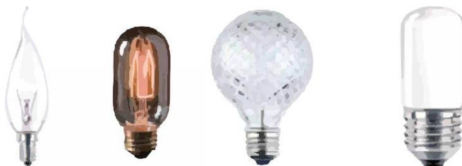
Figure 40 Low wattage decorative incandescent lamps. Left: Flicker-effect decorative swan-neck lamp, 3W, E14, 1000h, 230V. Middle: Two decorative incandescent lamps <11W. Right: Night light lamp, 11W, 230V, E27
