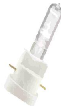
Figure 56 Ceramic MH lamp for theatres and studios (left), 250 W, 100V, 23000 lm (92 lm/W), 3200 K, 90Ra8, GZY9.5 base, Life to 50% failure 4000h. (Philips), Possible retrofit for 1000 W halogen lamp (75% energy saving). Right: Halogen lamp for professional spots 'Lock-it!'.
