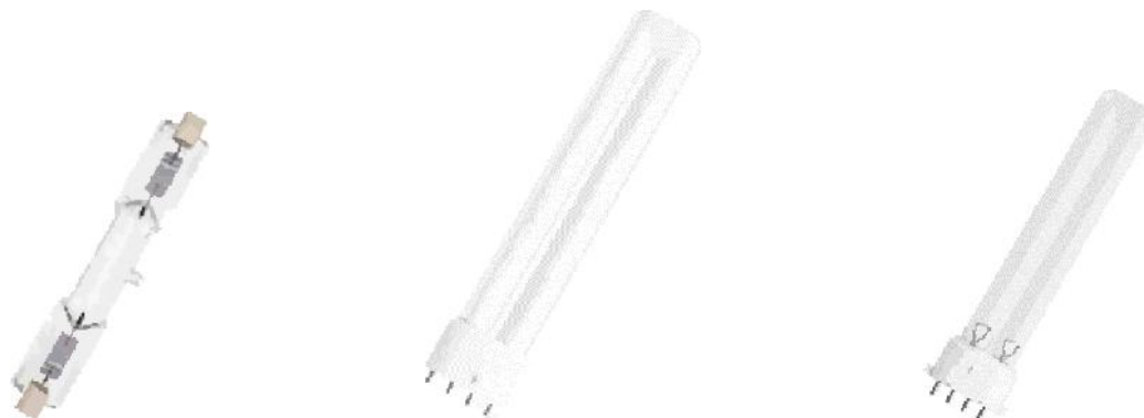
Figure 66 Examples of UV lamps. Left: Supratec Blacklight and blue light for industrial applications (18W, 57V). Middle: UV-A ('Blue') lamp, 45-61V, 7-18W. Right: UV-C germicidal ultraviolet lamps, 4-55W, disinfection without chemicals, low mercury content, long lifetime due to specific coating, ozone-free. dominant wavelength: 254 nm (OFR version)
