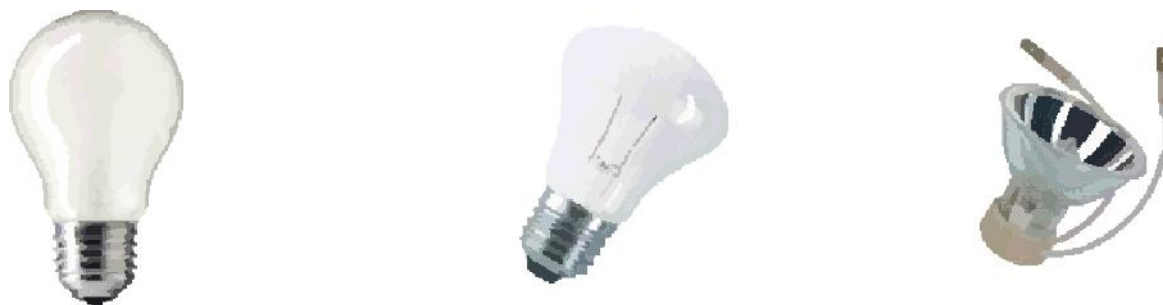
Figure 29 Traffic signalling lamps. Left: With B22 or E27 base. Range 40-60W, life 2000h, 230V or low voltage (12V, 24V, 48 V);
