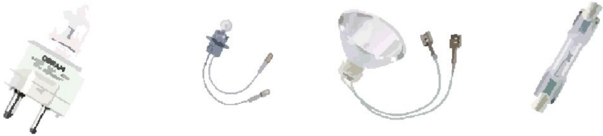
Figure 31 Current-controlled halogen lamps for airports. (30-45W, 430 lm, 6.6A, GY6.36, 1000-2000h) to (150W, 4000 lm, 6.6A, G9.5) for air-fields. Dimmable. Infrared radiation output that provides light in the worst of conditions. Halogen low-voltage lamps (double-ended, 100W, R7s, 6.6A, 2170 lm, 1000h) for current-controlled operation are used mainly in series-connected systems for airfield lighting.
