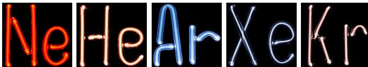
Figure 24 Originals colours produced by a cold cathode discharge tube ('neon tube') charged with respectively neon, helium, argon, xenon and krypton.
