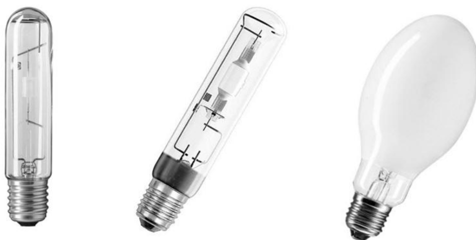
Figure 4: Example of lamps with socket type E40, typically used for lamps > 500 W (40 mm Mogul or Goliath Edison Screw, IEC 60061-1 standard sheet 7004-24).
