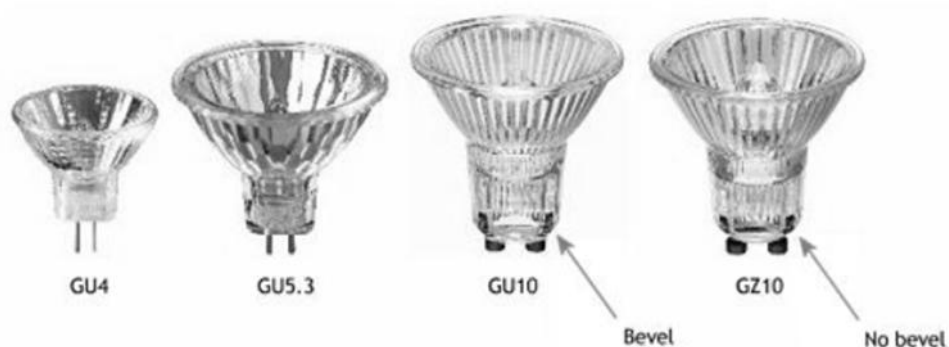
Figure 13: The most common halogen spots are either push fit (GU4 or GU5.3), low voltage type, or twist and lock (GU10 or GZ10) mains versions. The GU10 has a bevel around the base but the GZ10 has a square corner. This stops the GZ10 being used in a fitting designed for a GU10 but allows the GU10 to be used in either. (courtesy of: http://www.lightbulbs-direct.com/article/fittings-caps-and-bases/ )
