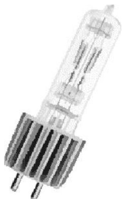
Figure 55 High Performance Lamp HPL halogen with arrangement of filament segments matched to ETC's "Source Four" spotlight family, 575-750W, 230..240V, 20-26 lm/W at 3050/3200K and 1500-400h, 11780..19750 lumen, 2 pin, d=19, 26 - 32 euros excl. VAT & shipping
