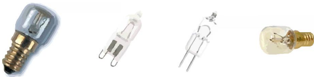
Figure 35 Oven and laundry drier replacement lamps. From left to right: 1) Incandescent microwave oven lamp, E14, 25 W, 230V. 2) Mains voltage halogen oven lamp, 25W, 260 lm, 2000h or 40W, 490 lm, 2000h (Class D). 3) Low voltage halogen oven lamp, 5-10-20W, G4, 12V, 60-140-320 lm/W. 4) Incandescent laundry drier lamp, 10W, 230V, E14
