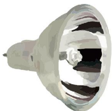
Figure 56 Ceramic MH lamp for theatres and studios (left), 250 W, 100V, 23000 lm (92 lm/W), 3200 K, 90Ra8, GZY9.5 base, Life to 50% failure 4000h. (Philips), Possible retrofit for 1000 W halogen lamp (75% energy saving). Right: Halogen lamp for professional spots 'Lock-it!'.
