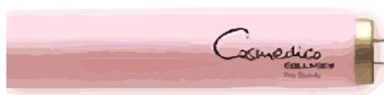
Figure 72 Collagen heat lamp, NOT an IR lamp. Collagen lamps are optimised to emit light in the visible red spectrum (picture: 100W, LFL form factor). They do not give tanning but only heat without side effects. Proposed now as retrofit for sunbeds originally bought for (UV) tanning. Unit price around 15-20 euros. (10 or 20 lamps per sunbed).
