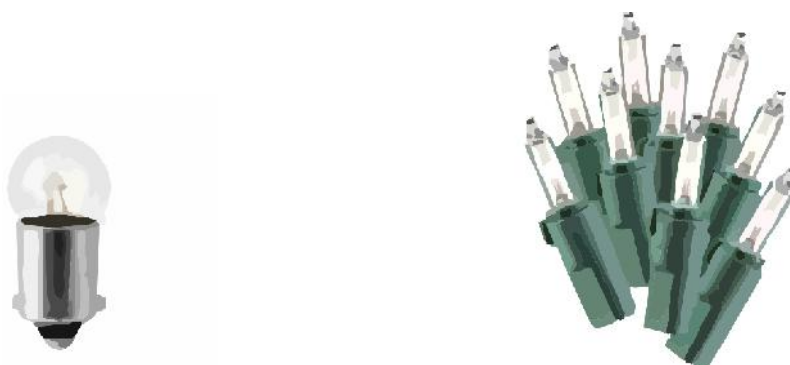
Figure 43 Mini-bulb lights (decorative). Left: Mini-bulb incandescent, 3.36W, 14V, incandescent, Miniature Bayonet (BA9s). Right: Mini string lights, incandescent mini-bulbs 50 or 100 lamps of 0.4W (20 or 40 W per string, no transformer needed) or LEDs 50 or 100 lamps of 0.1W (5 or 10 W per string, incl. LED driver/transformer).
