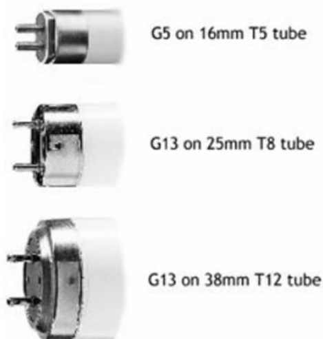
Figure 15: Fluorescent strips (LFL) generally have a two-pin fitting at both ends of the tube. Standard size T8 (25mm) and the larger T12 (38mm) tubes both use the G13 fitting. The smaller T5 (16mm) tubes use the G5 fitting with 5mm between the two pins. (courtesy of: http://www.lightbulbs-direct.com/article/fittings-caps-and-bases/ )
