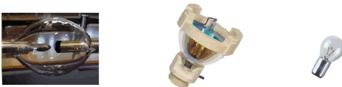
Figure 46 The full range of traditional projector lamps. Left: 15 kW xenon short-arc lamp used in IMAX projectors (source: Atlant at wikipedia.en). Diameter of the reactor bulb around 20cm. Middle: Xenon-arc reflector lamp 100-150W for video/ TV projection. Right: Low voltage, incandescent film projector lamp.
