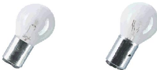
Figure 30 Train signalling lamps. Left: standard 12V, 6-20W, 600- 2000 – 6000h, B20d. Right: double filament (if 1st filament breaks the 2nd filament takes over), B15s (12V, 24V, 48 V);
