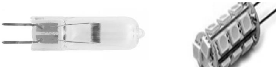
Figure 12: Miniature halogen capsule (left) and LED replacement (right) with GY6.35 type socket (low voltage use; 6.35 mm is pin distance).
