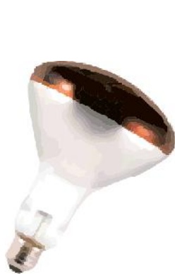
Figure 69 Infrared lamps. Left: Infrared incandescent lamp 100-375W, 230..240V, 1100 nm, E27, 30 °angle, 5000h, l=136, D=122 (OSRAM Siccatherm). Middle: Infrared halogen lamp 200-1000W, 230..240V, 1100 nm, R7s, position p15, lamp l=187.5, filament l=120 (OSRAM Halotherm). Right: Gold-coated IR heat lamp, as used for comfort heating (Dr. Fischer).
